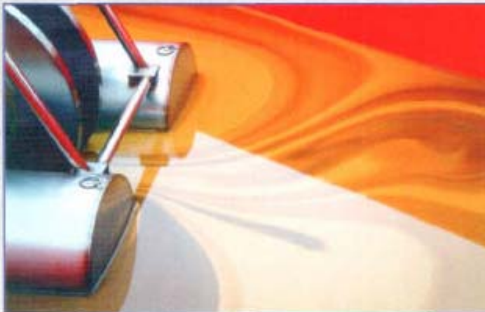
Discs inducing flow of pollutants to skimmer
